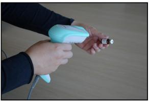
2. Pull the trigger to initiate scanning.
